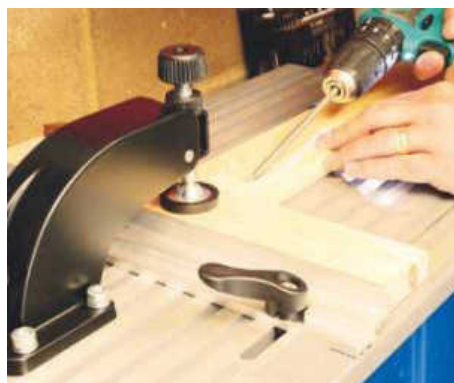
Once cut, the joints are screwed together in the normal manner
